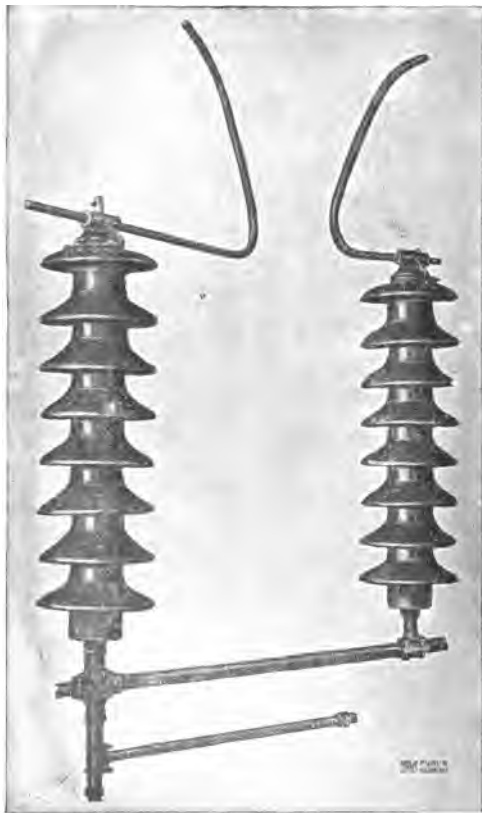
FIG. 232. Horn gap for 110,000-volt aluminum lightning arrester. One horn is connected to the line and the other to the ground, generally through an aluminum cell. The General Electric Co.
